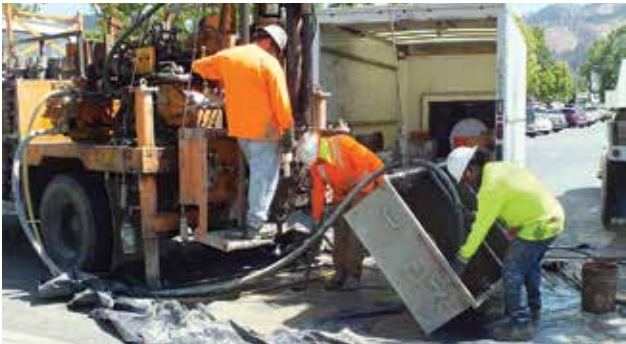
RGH Geotech workers perform exploratory 4-inch drilling and core sampling between the Berger Center and its parking lot. The June 7 test was recommended as part of a seismic study to determine the characteristics of ground the Berger sits on to verify the building is stable over the long term. It is a standard construction test. (Photo by John Williston)
